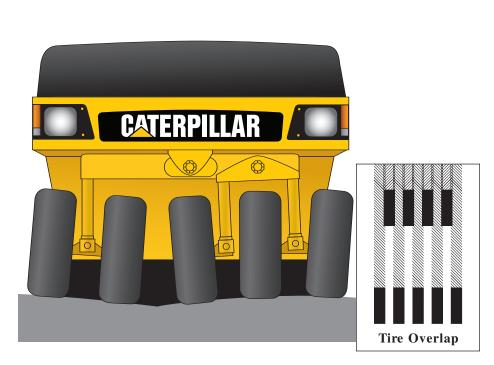
**Front and rear wheels paths** overlap 13 mm (0.5") to provide full-width coverage of 1743 mm (69") and 2134 mm (84") with 11-wheel option.
