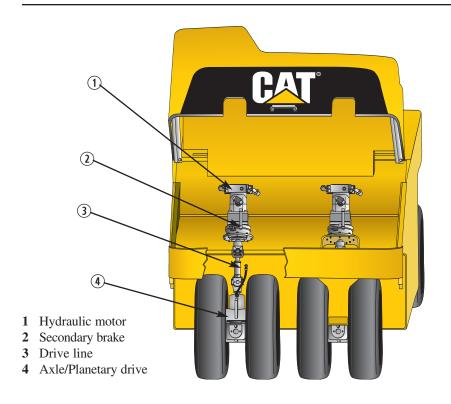
**Power transmission with drive line** provides smooth starts and stops – no chains are used.
