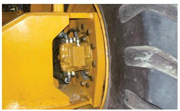
**FOUR-WHEEL PLANETARY DRIVE SYSTEM** The four-wheel Caterpillar planetary design system maximizes pushing power while allowing for a tighter turning radius and lower center of gravity.
