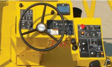
MAIN CONTROLS AT YOUR FINGERTIPS All of the commonly used functions are located based on real operator input. A manual push-button override allows the operator to run the elevator at max capacity without changing the preset running speed. This provides for quick catch up if a truck is delayed getting to the hopper.
