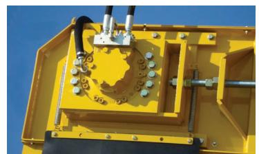
**DIRECT DRIVE MOTORS REDUCE NUMBER OF WEAR PARTS AND INCREASE RELIABILITY** The elevator is direct drive with two high-torque hydraulic motors, the conveyor is driven with one. There are no gearbox seals, bearings or fluids to worry about. The loop flush valve keeps the motor cool.
