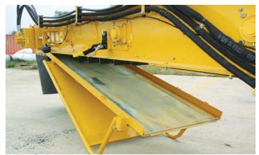
**CONVEYOR & ELEVATOR DROP OUT FLOOR** Clean out of the conveyor and elevator is made easy. Whether cleaning the machine or performing maintenance, this feature is sure to make the crew and service personnel jobs easier.
